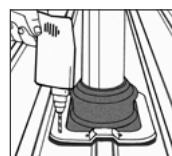
4. Fasten DEKTITE® with self-drilling screws or folding blind rivets.
